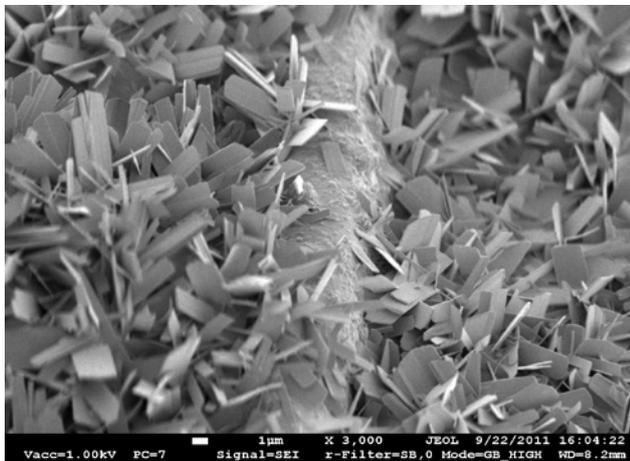
Fig. 4. Basalt fiber in the matrix of autoclaved aerated concrete (courtesy of VGTU).
