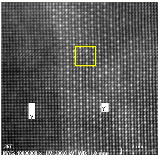
Fig. 7a. HRSTEM-HAADF image of the  $\gamma$  -  $\gamma'$  interface in Inconel 718 nickel-base superalloy for aeronautics and aerospace application.
