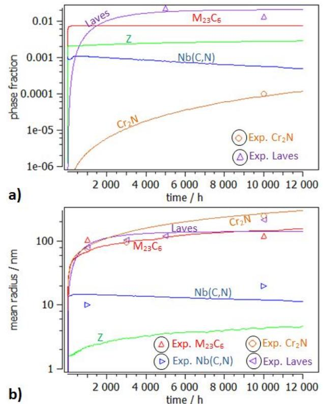
Fig.3. Experimental and calculated precipitates evolution in an advanced austenitic steel 22Cr25NiWCoCu (Sanicro25) during aging at 700°C for 10,000h. **a)** Phase fraction evolution and **b)** Precipitates mean radii evolution. (Courtesy of TUG)
