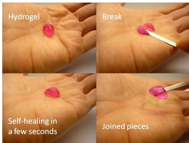
Fig. 5. Self-healing of supramolecular hydrogel (Courtesy of IK4-CIDETEC)
