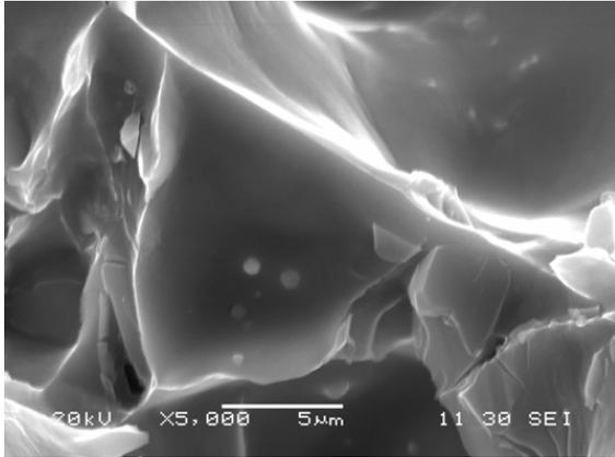
Fig. 1. AZ91 Magnesium alloy reinforced with submicron sized TiC particulates produced by SHS (Self propagating high temperature synthesis) (Courtesy of TECNALIA).
