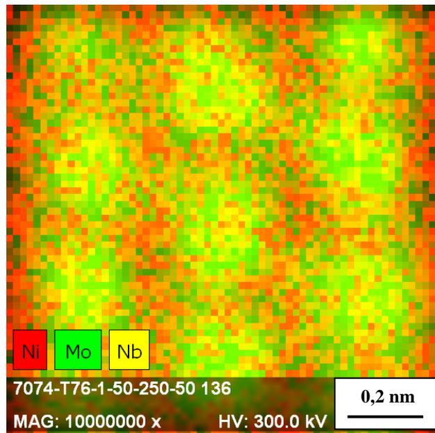
Fig. 7b. HRSTEM-EDX elemental maps of Ni, Mo and Nb in the  $\gamma'$  phase precipitated in Inconel 718 nickel-base superalloy. The image shows the enlarged scanned area marked by a yellow square in Fig. 7a.
